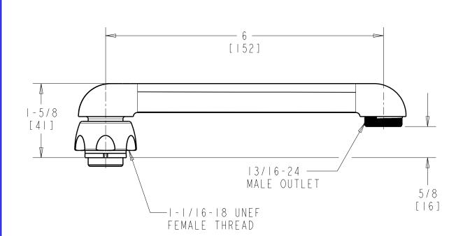
DIMENSIONS ARE IN INCHES AND [MILLIMETERS].
