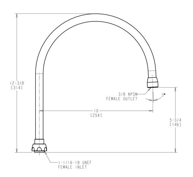
DIMENSIONS ARE IN INCHES AND [MILLIMETERS].
