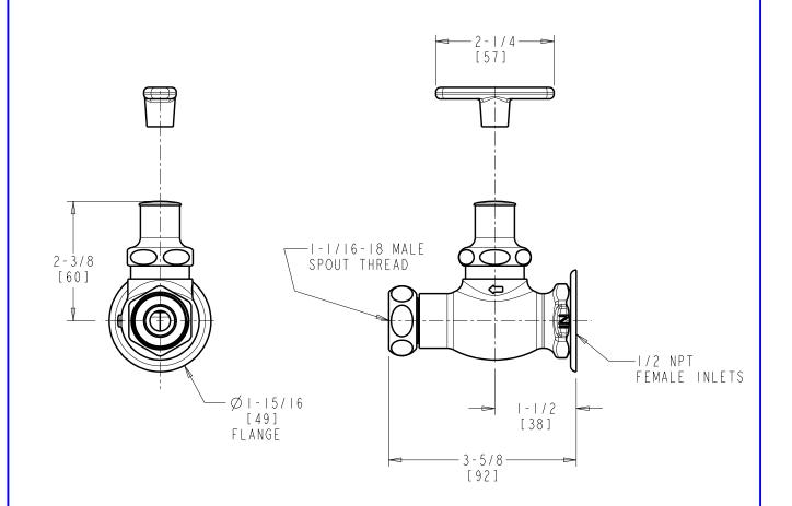
DIMENSIONS ARE IN INCHES AND [MILLIMETERS].
