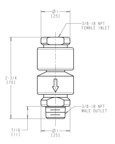
DIMENSIONS ARE IN INCHES AND [MILLIMETERS].
