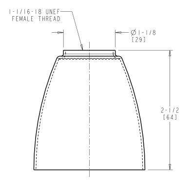
DIMENSIONS ARE IN INCHES AND [MILLIMETERS].
