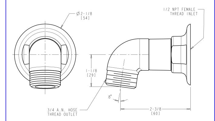
DIMENSIONS ARE IN INCHES AND [MILLIMETERS].
