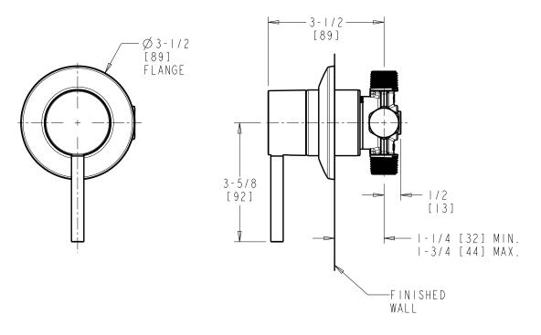
DIMENSIONS ARE IN INCHES AND [MILLIMETERS].
