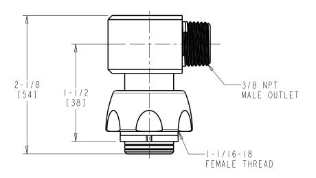
DIMENSIONS ARE IN INCHES AND [MILLIMETERS].
