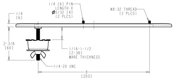
DIMENSIONS ARE IN INCHES AND [MILLIMETERS].
