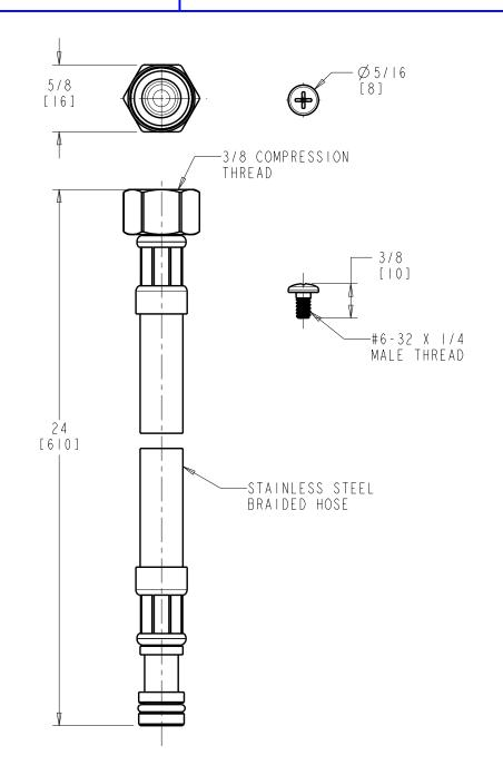
DIMENSIONS ARE IN INCHES AND [MILLIMETERS].
