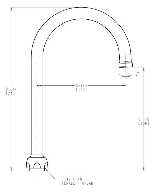
DIMENSIONS ARE IN INCHES AND [MILLIMETERS].
