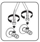
Insert the filter screen gaskets into the supply stops. Attach the 3/8" female compression supply hoses from the mixer to the supply stops. Use a wrench to tighten the nuts to the supply stops.
