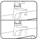
4. Remove outlet and flush lines.
