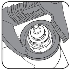
2. Loosen cartridge assembly using channel locks.
