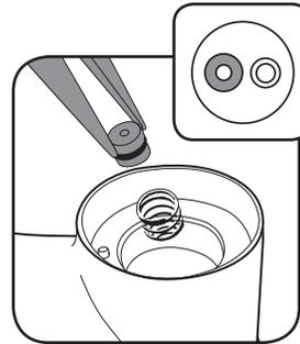
4. Remove hot orifice seat using needle nose pliers. The hot orifice seat is on the left.
