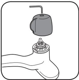
1. Using wrench, remove hex screw and handle. Depress actuator stem to purge any residual pressure.
