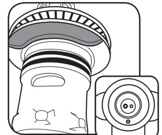
5. Align mounting pin to groove in brass nut when replacing cartridge assembly. Pin orientation should face front.
