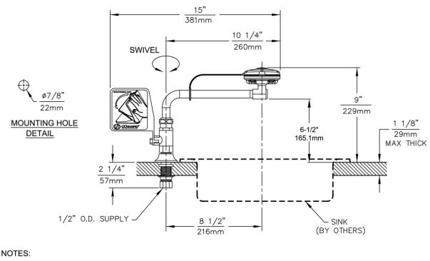
1. THE ANSI Z358.1-2009 STANDARD SPECIFIES EYEWASH NOZZLE HEIGHTS TO BE 83.8cm (33 IN.) TO 114.3cm (45 IN.) ABOVE THE FLOOR. CENTERLINE OF EYEWASH HEADS MUST BE 15.2cm (6 IN.) MIN. AWAY FROM WALL OR NEAREST OBSTRUCTION.
