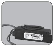
Note the top number on the sensor label. Use the chart below to determine the current default mode of the faucet. Discard the sensor.
