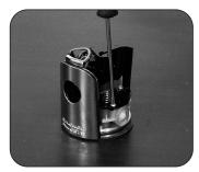
4. Loosen the screw on the battery holder. You do not have to remove it completely.
