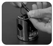
9. Connect the sensor to the faucet. Tuck wires into the faucet body.
