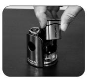
Remove the battery or the AC adapter.
