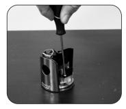
8. Tighten the screw on the battery holder.
