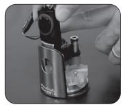
7. Insert the Bluetooth® sensor and battery holder.
