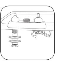
Attach water inlet hoses and tighten.
