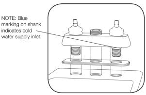
Attach washers and locking nuts and tighten.
