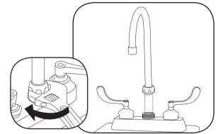
7 Remove outlet, flush lines for at least 2 minutes, and reinstall outlet.
